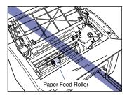
• The area around the output tray becomes very hot during printing and directly after printing. When you are collecting paper from the output tray or clearing a paper jam, be careful not to touch the area around the output tray.
